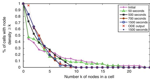
**Fig. 11** RWP simulation using initial density conditions from the trace (solid lines), and simulation using the output of the ODE framework as the initial density conditions (dashed lines)
