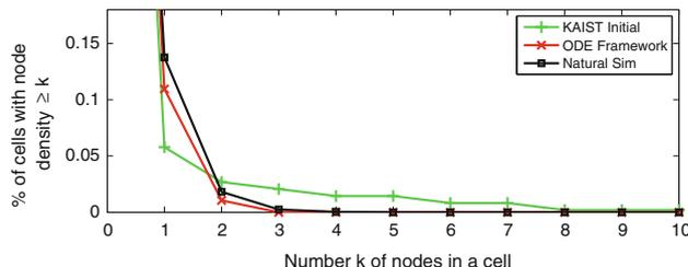
**Fig. 8** Initial spatial node density distribution for the KAIST trace, simulated final density distribution using the Natural mobility regime and the respective steady-state density distribution using the proposed ODE framework applied to the Natural mobility regime
