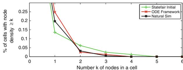
**Fig. 10** Initial spatial node density distribution for the Statefair trace, simulated final density distribution using the Natural mobility regime and the respective steady-state density distribution using the proposed ODE framework applied to the Natural mobility regime
