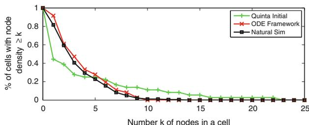
**Fig. 6** Initial spatial node density distribution for the Quinta trace, simulated final density distribution using the Natural mobility regime and the respective steady-state density distribution using the proposed ODE framework applied to the Natural mobility regime
