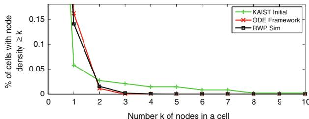
**Fig. 7** Initial spatial node density distribution for the KAIST trace, simulated final density distribution using the RWP mobility regime and the respective steady-state density distribution using the proposed ODE framework applied to the RWP mobility regime
