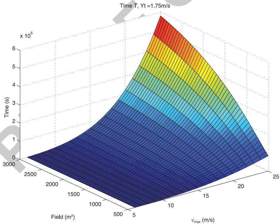
(b) Warm-up times for speed decay of  $Y_t = 1.75\text{ m/s}$
