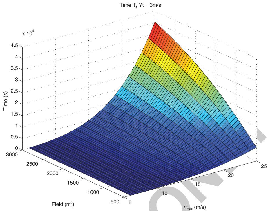
(a) Warm-up times for speed decay of  $Y_t = 3\text{ m/s}$
