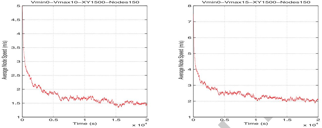
Figure 1. Speed decay under the random waypoint model
