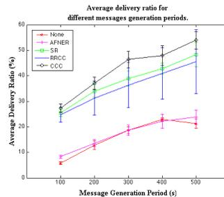
Figure 2: Message delivery ratio as a function of the message generation period (Epidemic routing, buffer size of 1000 Kbytes, transmit speed of 2.5 Mbps and RWP mobility model).
