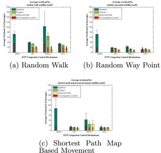
Figure 5: Average overhead per congestion control mechanism for different mobility models (transmit speed of 2.5 Mbps, buffer size of 500 Kbytes and message generation period of 300 s).
