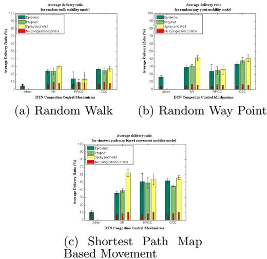
Figure 3: Average delivery ratio for each congestion control mechanism using different mobility models (transmit speed of 2.5 Mbps, buffer size of 500 Kbytes and message generation period of 300 s).
