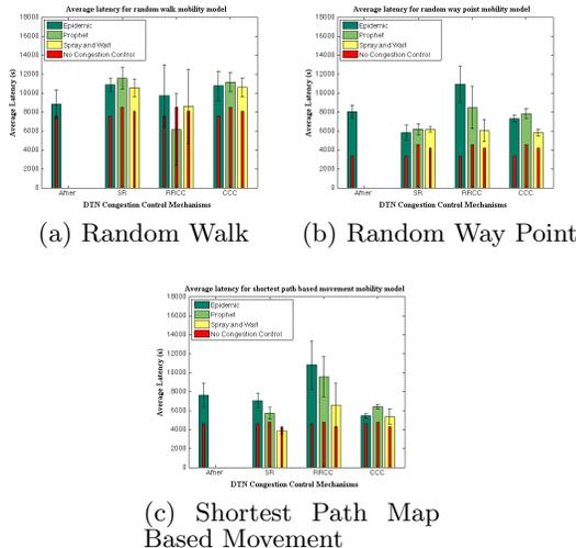
Figure 4: Average latency per congestion control mechanism for different mobility models (transmit speed of 2.5 Mbps, buffer size of 500 Kbytes and message generation period of 300 s).
