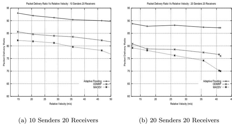
Figure 1: Packet Delivery Ratio as a function of Node Mobility
