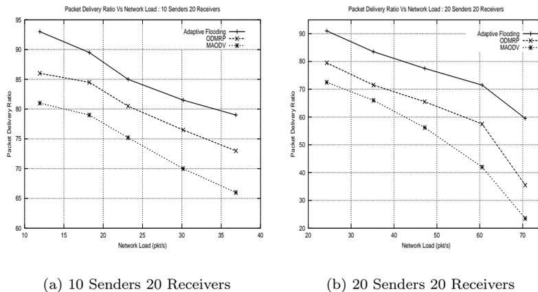
Figure 3: Packet Delivery as a function of Network Load
