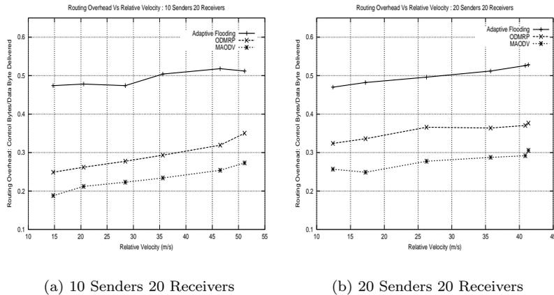
Figure 2: Routing Overhead as a function of Node Mobility
