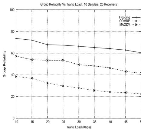
Figure 14: Group reliability as a function of traffic load
