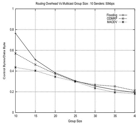
Figure 7: Routing overhead as a function of group size
