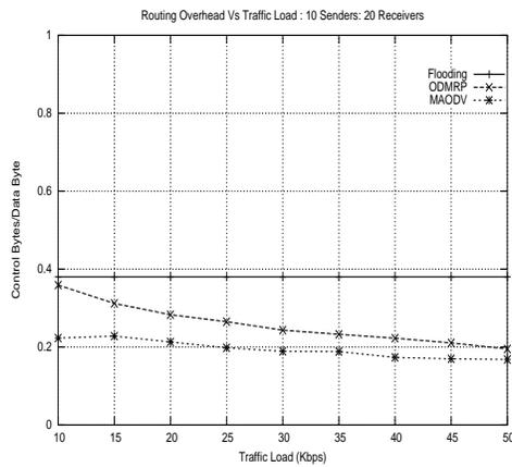
Figure 13: Routing overhead as a function of traffic load
