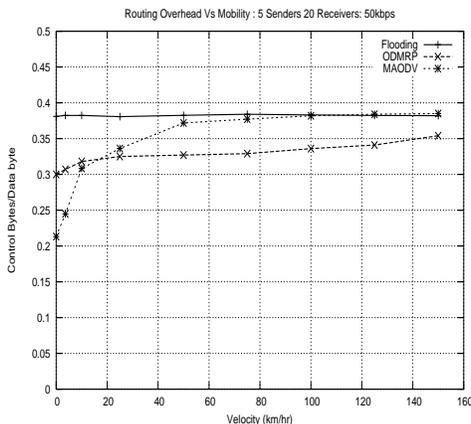
Figure 4: Routing overhead as a function of node mobility
