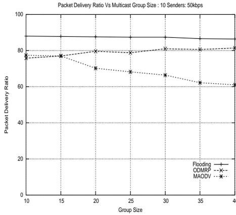
Figure 6: Packet delivery ratio as a function of multicast group size
