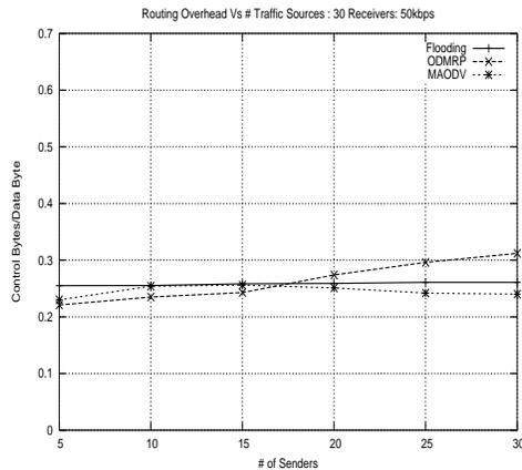
Figure 10: Routing overhead as a function of traffic sources
