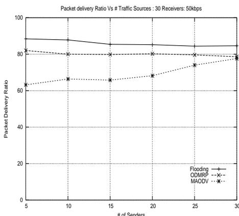
Figure 9: Packet delivery ratio as a function of number of traffic sources
