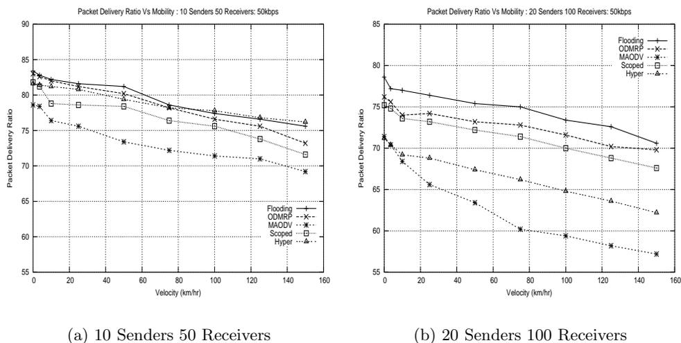
Figure 15: Packet delivery ratio as a function of node mobility
