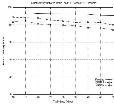
Figure 12: Packet delivery ratio as a function of traffic load
