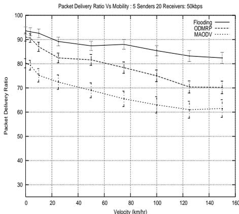
Figure 3: Packet delivery ratio as a function of node mobility
