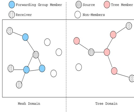
Figure 2: Flooding-based interoperability: initial route setup across two routing domains.
