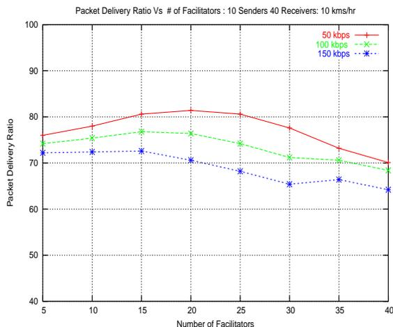
Figure 14: Packet delivery ratio versus number of facilitators with varying traffic load
