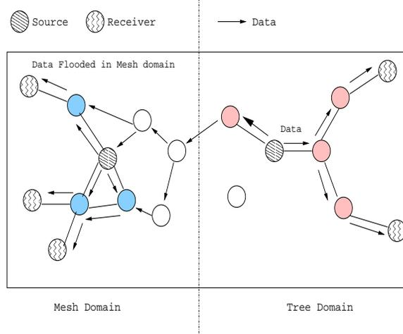
Figure 3: Flooding of data in mesh routing domain
