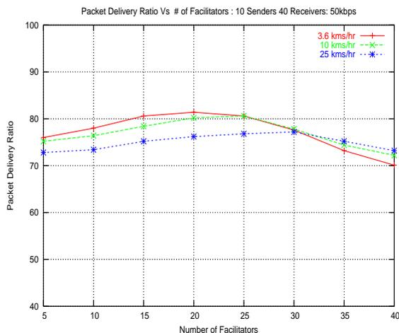
Figure 13: Packet delivery ratio versus number of facilitators for different node mobility
