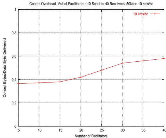
Figure 12: Control overhead versus number of facilitators
