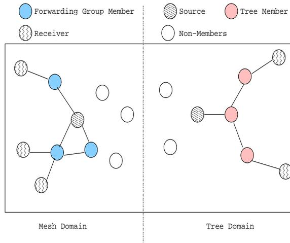
Figure 4: Facilitator-assisted interoperability: initial route setup across two routing domains
