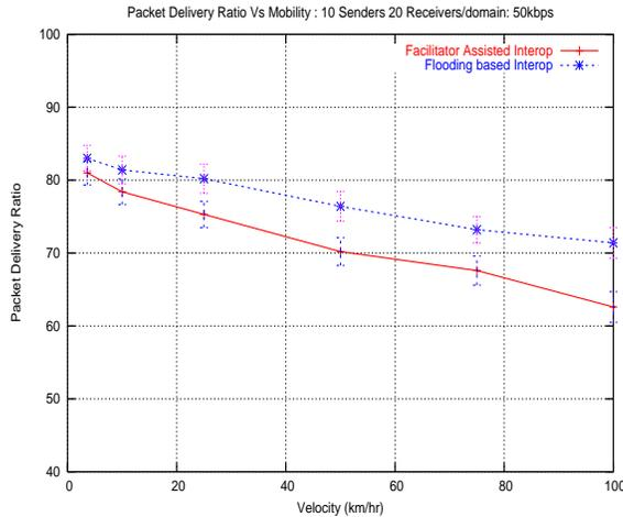
Figure 9: Packet delivery ratio as a function of node mobility
