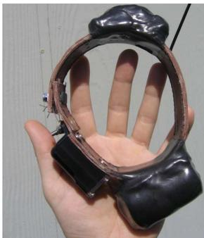
Fig. 3. Picture of deployed CARNIVORE node. The CARNIVORE electronics are above, D-cell battery and VHF beacon are lower-right, and a timed drop-off (SirTrack [16]) is lower-left. Components were assembled by Telemetry Solutions.
