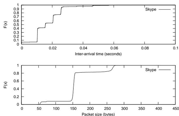
Fig. 5. Cumulative distribution function plots showing packet inter-arrival time and packet size. There are around 5 discrete inter-arrival times and 3 discrete packet sizes.
