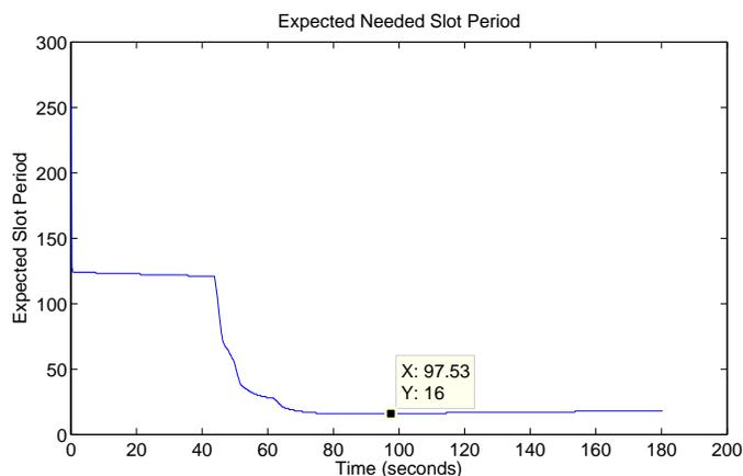
Fig. 6. Forecaster output: prediction of slot period required to service a flow that produces lowest delay and wasted slots. Given that the slot duration was set at  $638.125\mu s$ , a slot period of 16 corresponds to  $10.210ms$  and this is exactly the inter-arrival time indicated by the lowest dark cluster in the top plot of Figure 5.
