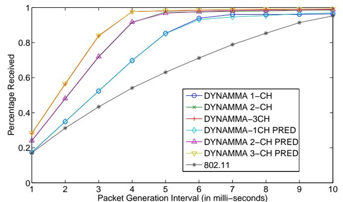
Fig. 3. Average delivery ratio of IEEE 802.11, DYNAMMA, and DYNAMMA-PRED.
