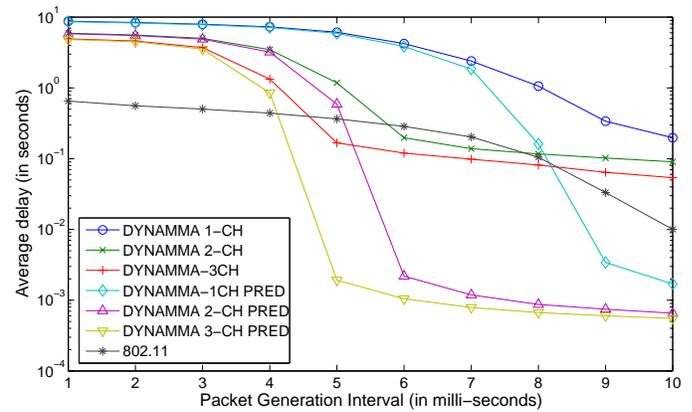
Fig. 2. Average queuing delay of IEEE 802.11, DYNAMMA, and DYNAMMA-PRED.
